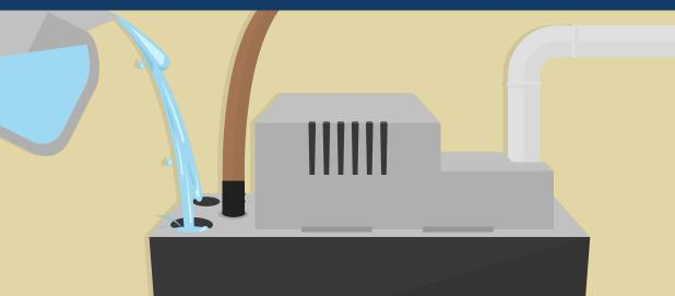
A common cause of a leaky air conditioning unit is a broken condensate pump. To be certain that it is the condensate pump that is causing the problem, pour some water into the drain pan. If the excess water is not pumped out, then the condensate pump is broken.
